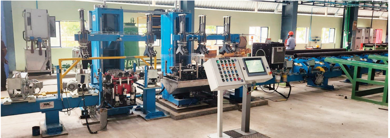
MAC's Spin-the-Tube system operating in a tube mill.
