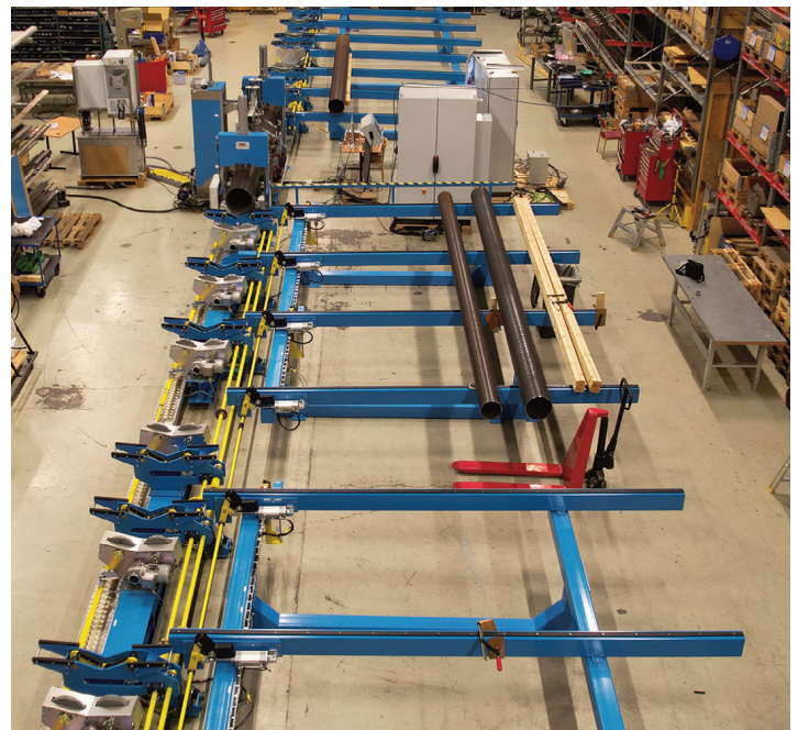
Spin-the-tube conveyor line is shown at left, incoming feed racks in center.
