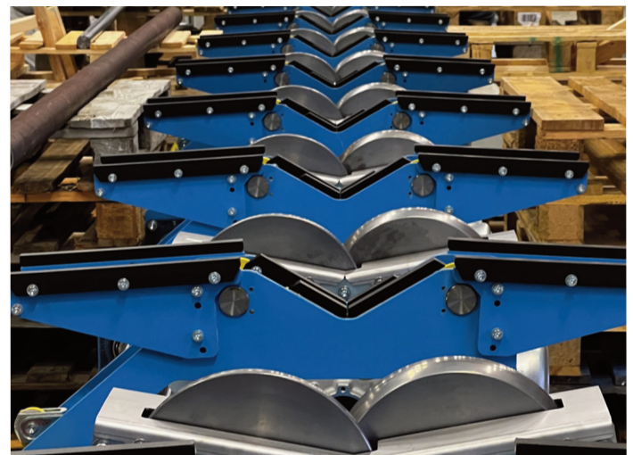
Rotating disks drive and spin the tubes through the test, maintaining the correct pitch.
