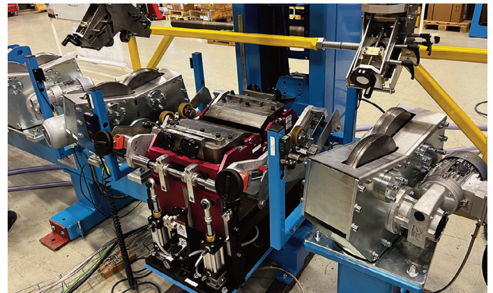
Magnetic Flux Leakage tester to detect through drilled holes.
