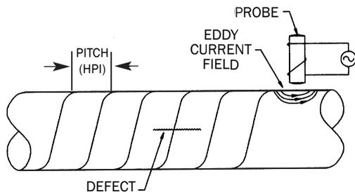
*To be consistently detected, the defect length must be greater than the helical pitch (HPI) of inspection. The HPI is a function of the probe's rotational speed and the throughput speed of the test material.*
