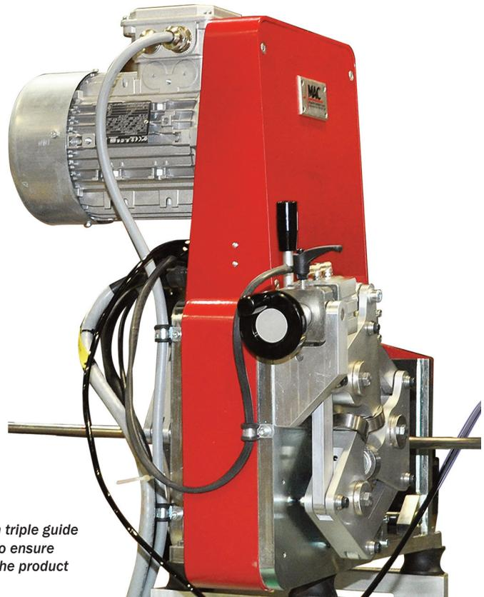
*Rotomac<sup>®</sup> 38mm with triple guide rolls at entry and exit to ensure proper positioning of the product*
