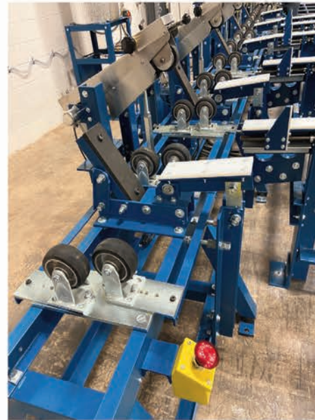
Model 620H Heavy-Duty Input Idler Section with load guides and extended drives
