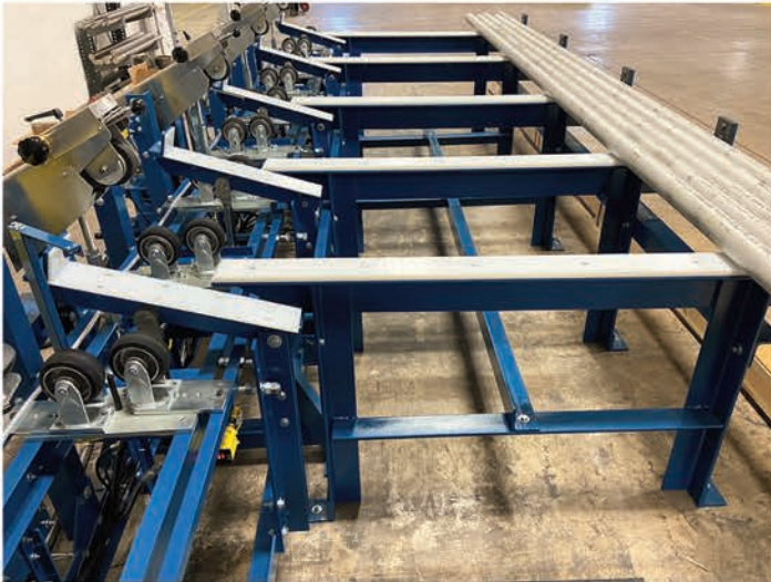
Model 188 Unloader in mid-cycle on heavy-duty output idler section with storage rails
