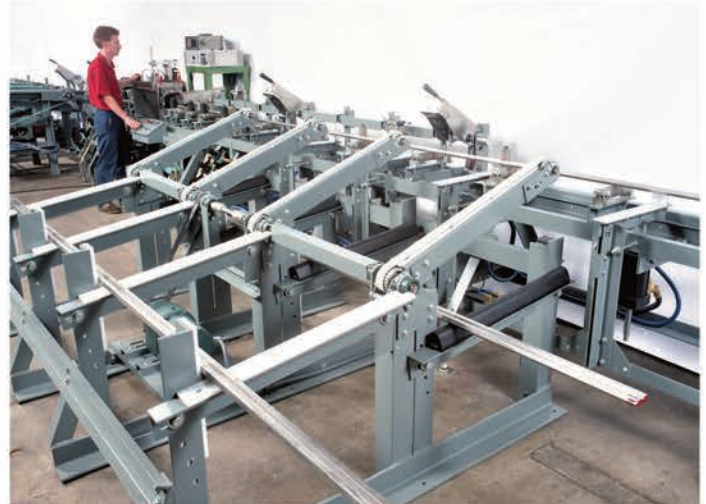
Model 77 Straight Through Tester with automatic loader and unloader shown with hex bar
