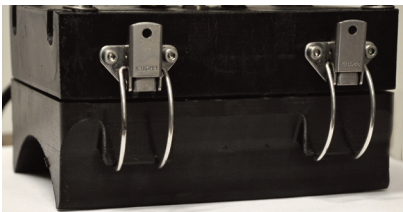
Customized, exchangeable test shoe and captive water chamber array head
