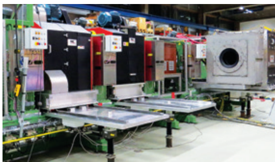
Magnetic Analysis Corp's 500mm UT/MFL test system for large diameter pipe
